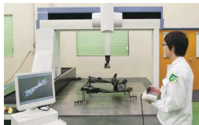
非接触3次元測定器 設計基準と部品精度にズレがないかを徹底的にチェックし、完成品の精度を高めます。 Non-contact 3D measurement machine We increase the accuracy of finished products by thoroughly checking them against the design standards to ensure that there are no errors in the part's accuracy.
