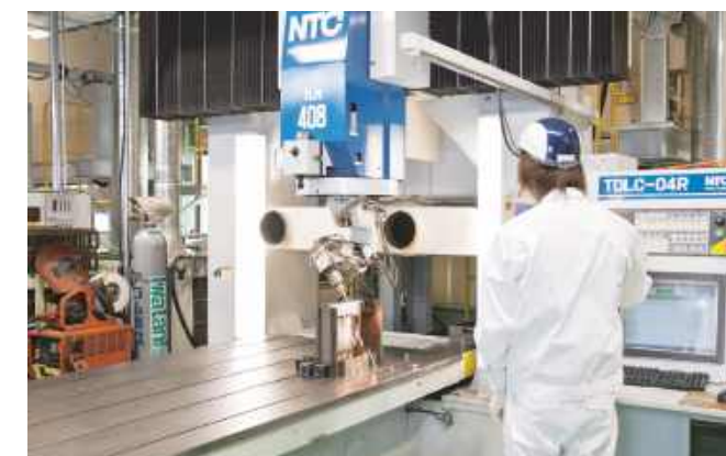
自動3次元レーザー加工機 切断と溶接を1台でこなし、より精密なプロトタイプを製作します。 Automatic 3D laser processor The processor is used for cutting, welding as well as for developing and manufacturing prototypes with more precision.
