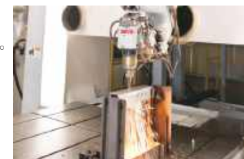
自動3次元レーザー加工機 切断と溶接を1台でこなし、より精密なプロトタイプを製作します。 Automatic 3D laser processor The processor is used for cutting, welding as well as for developing and manufacturing prototypes with more precision.
